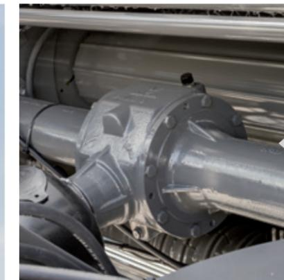
The Powersplit gearbox equally divides and transfers power to drive the rotor unit on one side and the roller drives on the other, reducing the overall power requirements by simplifying the drivelines. With the upgrade to the 1,000 rpm gearbox, you will receive:
