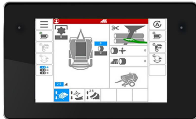
The **Bale Control Terminal**, supplied as standard, gives the operator a great overview of the baling process and includes a range of intuitive functions. The high-definition touchscreen features a modern working display with improved operating efficiency.
