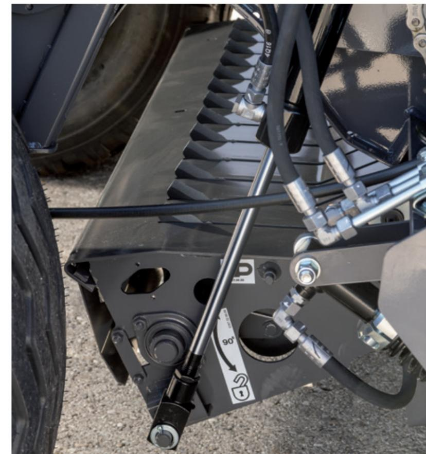
The first stage of Hydroflexcontrol allows movement of the front part of the feed chamber floor and will automatically prevent up to 80% of potential blockages and will keep you going without unnecessary downtime.
