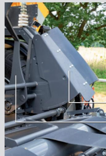
In addition to the transfer arm, the design features two active guiding plates on both sides of the baler clearly directing the bale to the centre of the wrapper plate allowing for a faster and more secure transfer cycle. For added safety in hillside conditions the unique slope transfer mode allows for the transfer arm to move more slowly while the wrapper ring is lifted higher to receive the bale. This ensures that the bale will be securely delivered to the wrapper even in sloping terrain.
