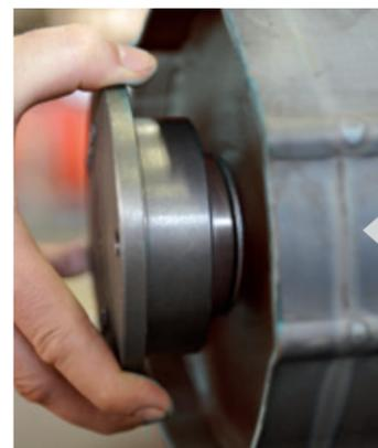
The bale chamber can experience extreme loads with forces from all directions. The clever bearing housing design allows some movement of the rollers to eliminate major axial loads occurring during operation.
