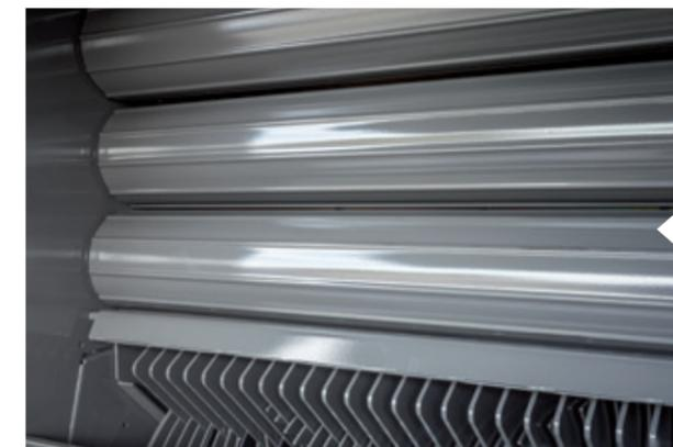
The roller support bearings in the bale chamber feature new scrapers, efficiently removing debris and moisture from the roller bearings and keeping the outside panels clean.
