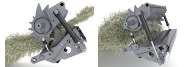
In the event of a blockage the operator can easily open the feed table floor and lower the knives at the same time to provide enough space for material to pass through.
