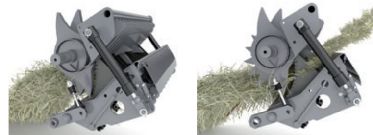
The patented protection system prevents peak loads from turning into blockages by a gentle lowering of the floor which is suspended on rubber blocks or steel springs, depending on the model.
