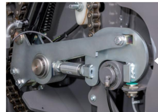
The simple, fast and efficient mechanical tail-gate locking device is now enhanced with pressure sensors on both sides and features left-right indication allowing the operator to monitor the outer layers of bale.
