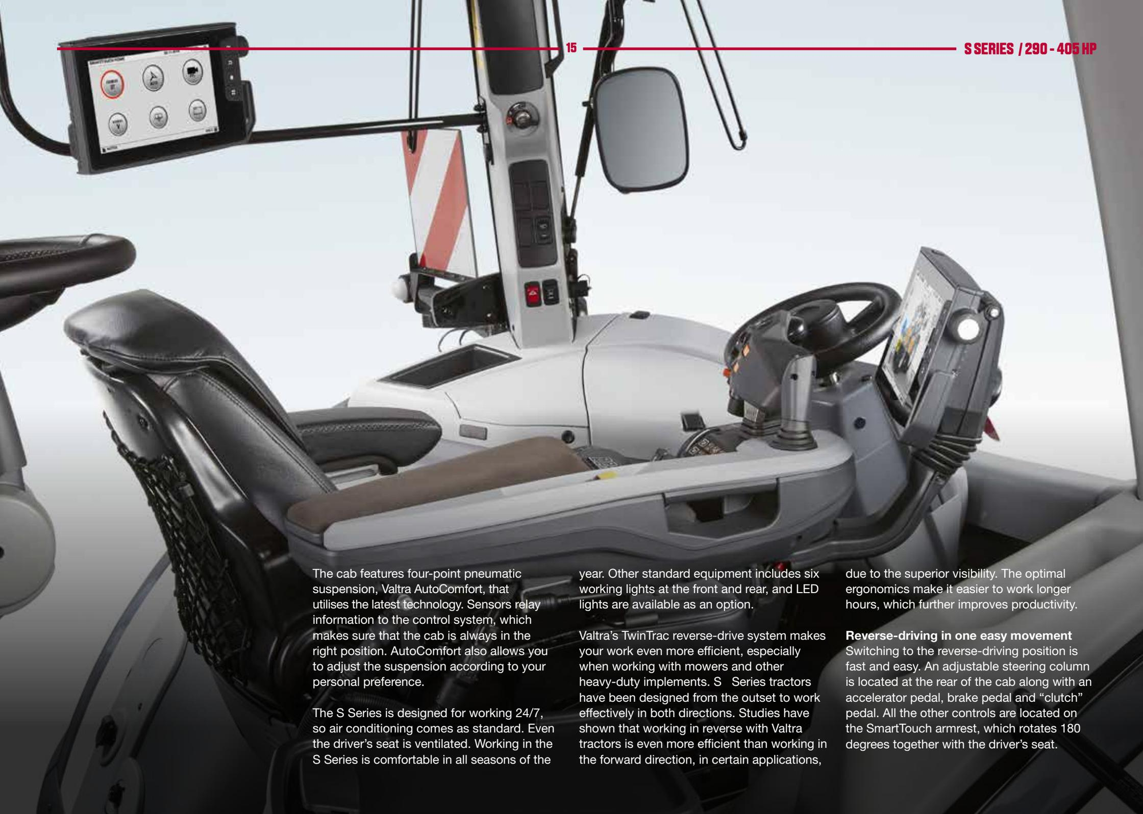
The cab features four-point pneumatic suspension, Valtra AutoComfort, that utilises the latest technology. Sensors relay information to the control system, which makes sure that the cab is always in the right position. AutoComfort also allows you to adjust the suspension according to your personal preference.
