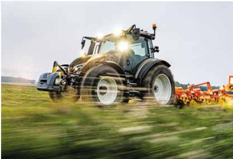
As the powerhouse of Valtra tractors with 70 years of experience, AgcoPower compact engines offer great power and torque feature. The compact 4.4 l engine with small dimensions enable a low bonnet with great visibility. The all-in-one engine after-treatment system cleans
