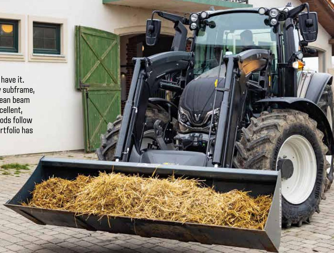
1. Modern, minimalist beam design with enclosed pipe work
