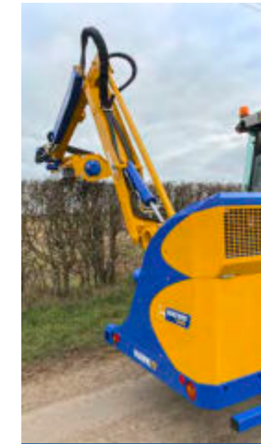
Oil cooler as standard High level keeping clear of any cutting debris.
