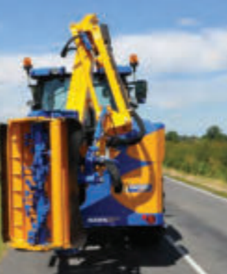
Transport bracket Supplied as standard for fast travelling on the road.
