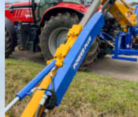
Steel hose covers Adding additional protection to drive motor houses.
