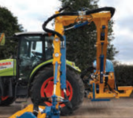
Telescopic 3rd arm on 6.0T and 6.5T models Gives increased flexibility.
