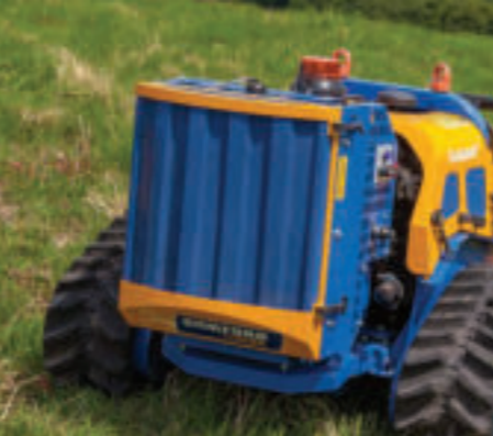
Radiator cooler cover Hinged cooler guard for easy access.
