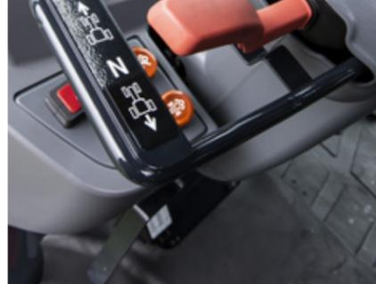
Electro-hydraulic shuttle lever on MF 1700 M models to improve comfort
