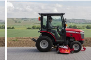
A new, improved 152 cm wide mower deck is equipped with three blades and offers cutting heights from 20 mm to 115 mm, adjustable in eight steps from the seat, as well as up to 150 mm of ground clearance.
