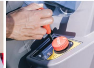
Well positioned hand throttle lever
