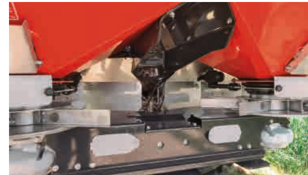
One electric actuator to control the application rate
