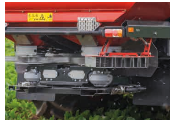
Border spreading - spreading to the border with the ExactLine
