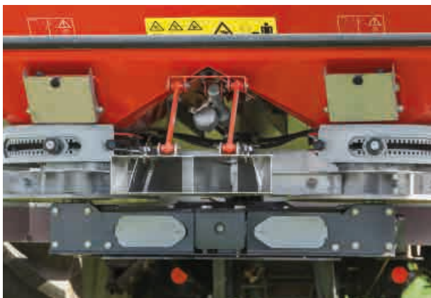
One-sided border spreading - spreading from the border with the border spreading plate
